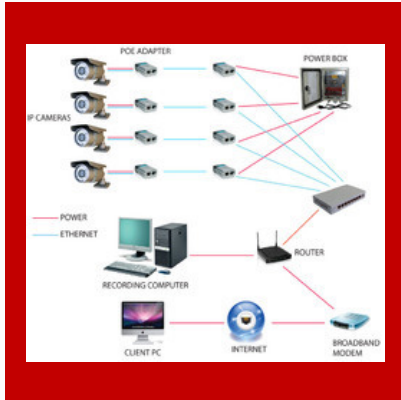
IP CCTV Camera System
